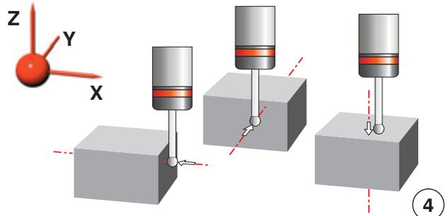
**Angle measurement on the X-Y plane (5)**
