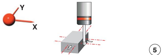
**Angle measurement with respect to the X-Z and Y-Z planes (6)**
